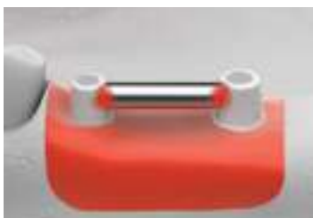
Fabrication of burn-out cylinder and plastic bar in preparation for wax-up.
