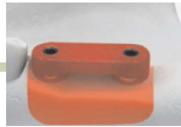
Fabricate the positioning jig
