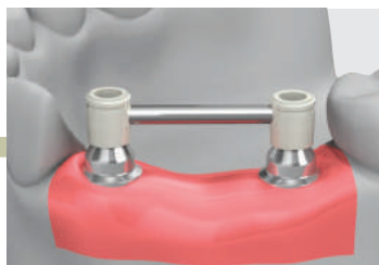
Connect the plastic bar in the middle of trimmed Screw Abutment to help support the wax pattern. Wax pattern may have shrinkage.
