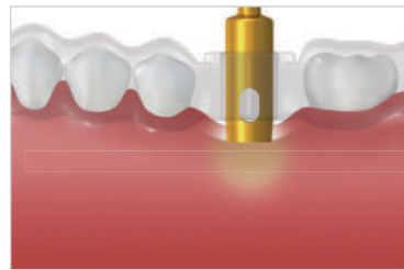
Tissue Punch FTP45 (1000rpm/30~45N-cm with irrigation)
